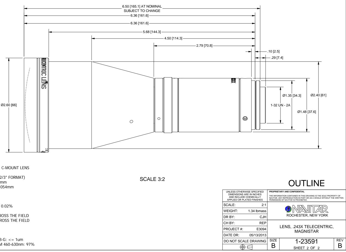
**BI-TELECENTRIC 0.243X F/8 C-MOUNT LENS** MAGNIFICATION: 0.243X IMAGE DIAGONAL: 11 mm (2/3" FORMAT) WORKING DISTANCE: 103.3mm BACK FOCUS DISTANCE: 39.054mm WORKING F/#: 8 SYSTEM F/#: F/6.5-F/22 **TELECENTRICITY: 0.04°** F TAN-THETA DISTORTION: 0.02% FIELD DEPTH: 11mm MTF: >50% @70lp/mm ACROSS THE FIELD CTF: >62% @70lp/mm ACROSS THE FIELD IMAGE NA: 0.062 OBJECT NA: 0.015 C-MOUNT LAT. COLOR R-G: <= 1um, B-G: <= 1um AVG. TRANSMITTANCE FROM 460-630nm: 97%
